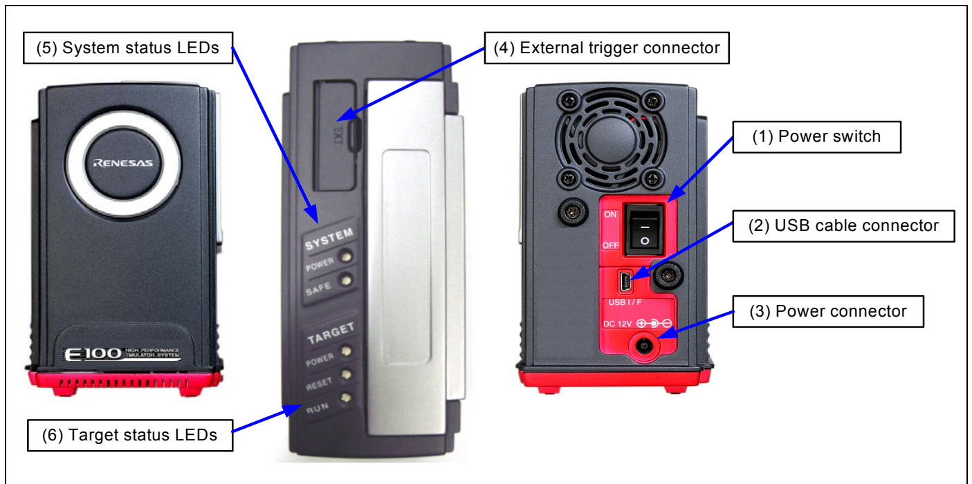
Figure 1.2 Names of each part of the emulator
